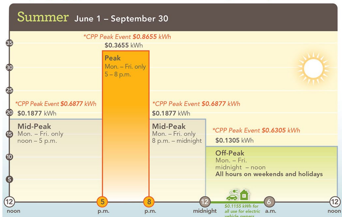
Figura 13: Esquema Critical Peak Pricing 47
